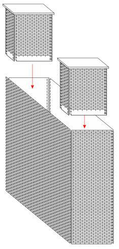
Insert posts into the pier making sure that they are aligned well. Misalignment at this stage can cause the parapet to not register correctly to the pier.
