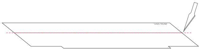
Cut both deck panels LCC 70-87 along the marked line for the single version of the bridge.
